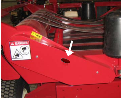
Figure 6.3 Other lubrication 2 (through the hole in the guard)
