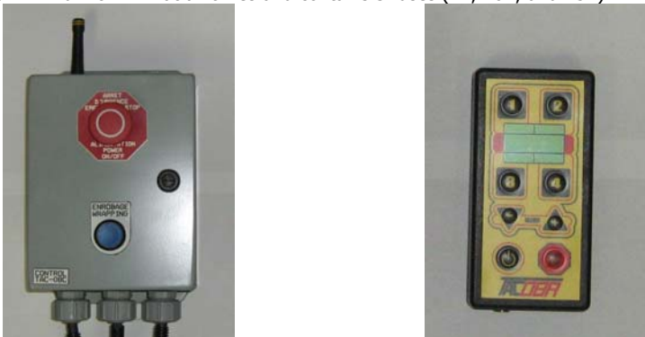
Figure 5.1 TAC-08 remote control (right) and TAC-08C receiver (left)
