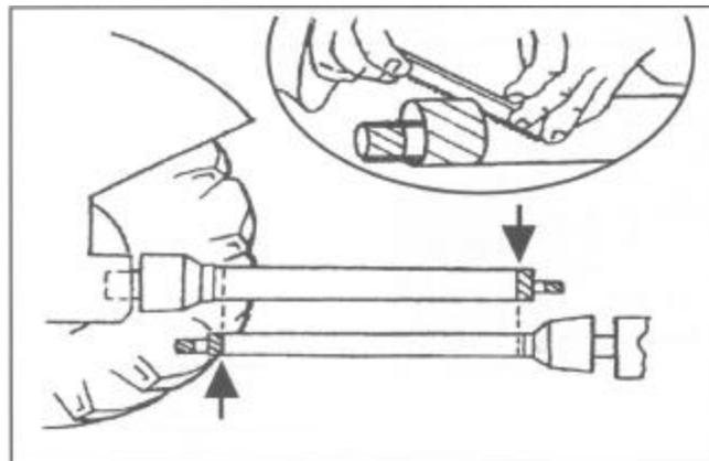
**CAUTION:** Do not shorten more than necessary. Shorten the metal tubes and guards by the same amount and round off all sharp edges. Grease the metal tubes before assembly.
