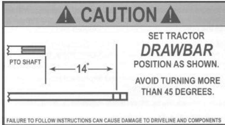
The tractor's drawbar must be set at a distance of 14" from the end of the P.T.O. shaft to the center of the drawbar pin hole. This distance is standard for P.T.O. drives and will maintain a proper relationship for driveline angles and help improve the life of the driveline.
